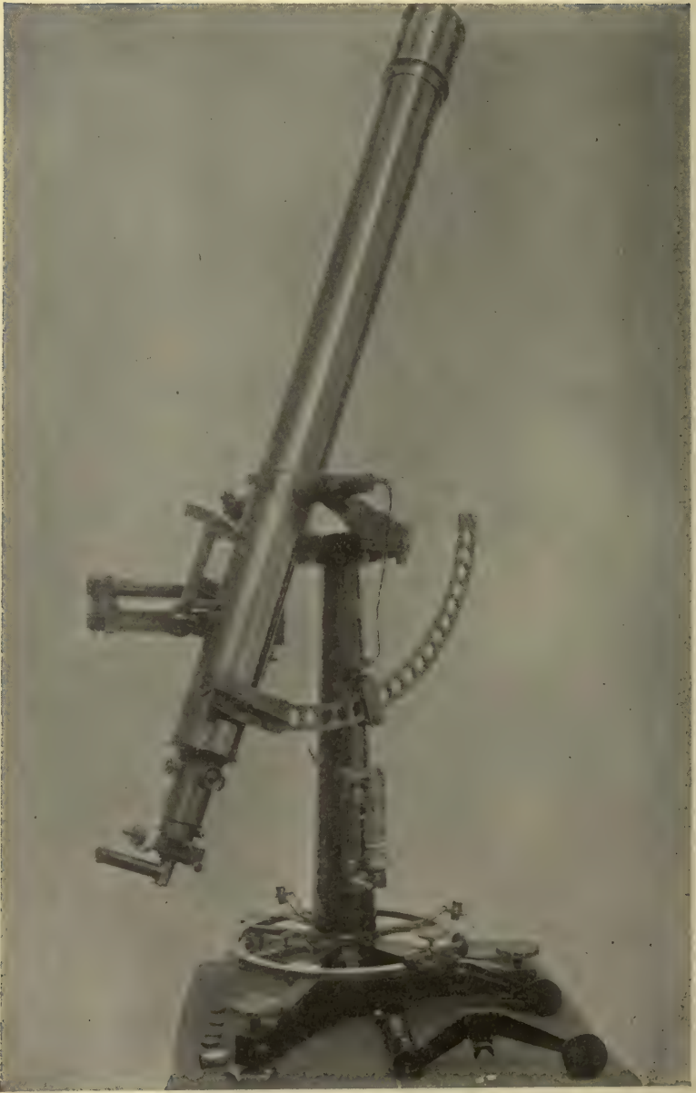
FIG. 52. Zenith Telescope. (Coast and Geodetic Survey.)
